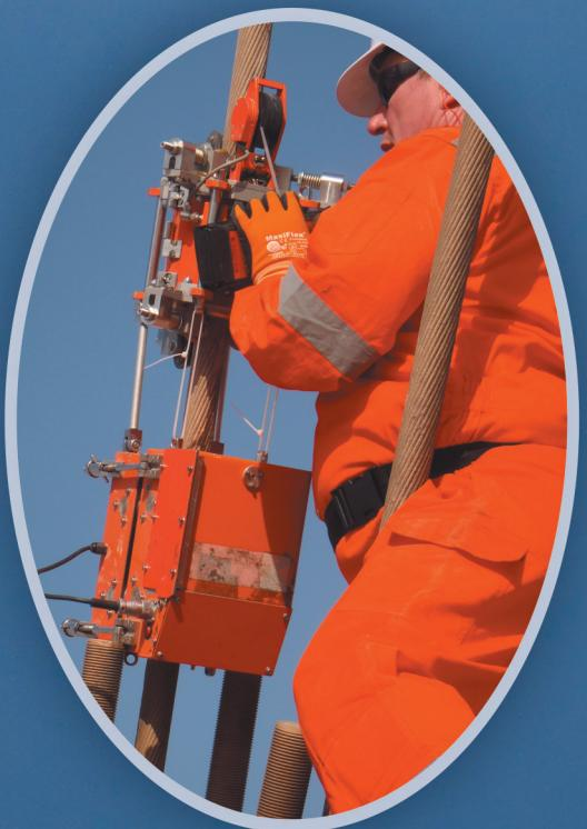
Flare stacks can be decades old, and guy ropes, operating in a sedentary environment are prone to continuous deterioration that includes corrosion and degradation in wires and strands. Continuing their safe operation requires accurate and objective inspection.
