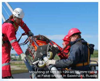
Besides inspection of bridge cables INTRON PLUS can non-destructively inspect wire ropes of different application onshore and offshore. Our services also include inspection of above storage tank floor and steel cord conveyor belts.
