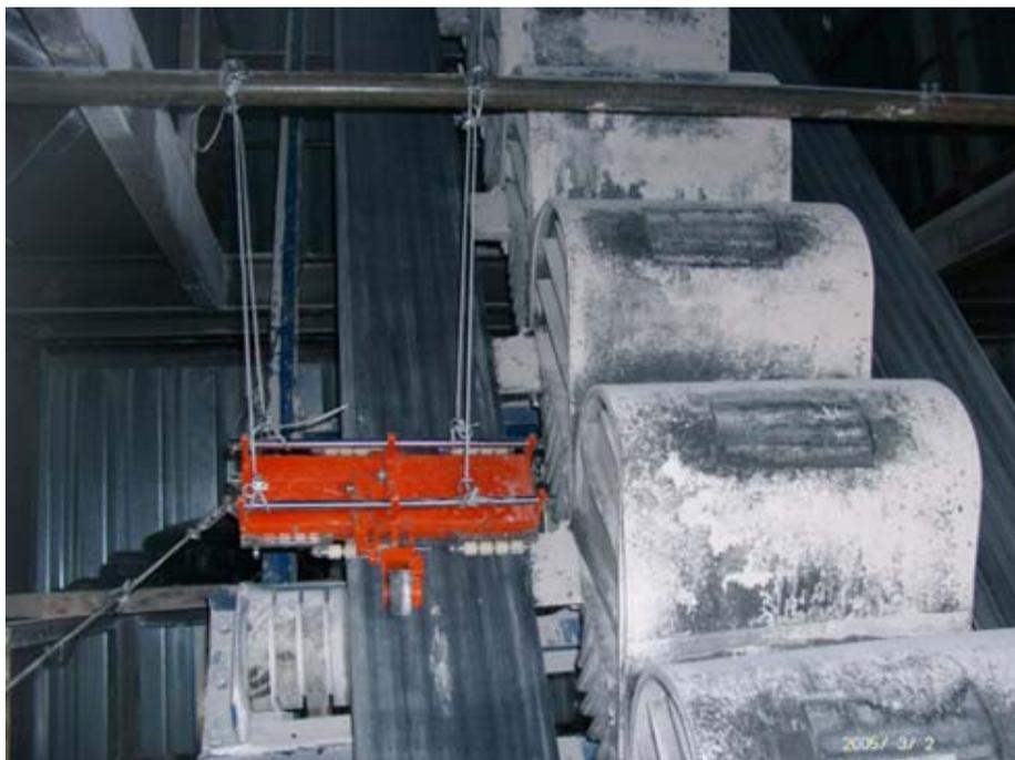
Fig. 6: The INTROCON scanner positioned on the Pocketlift conveyor belt.
