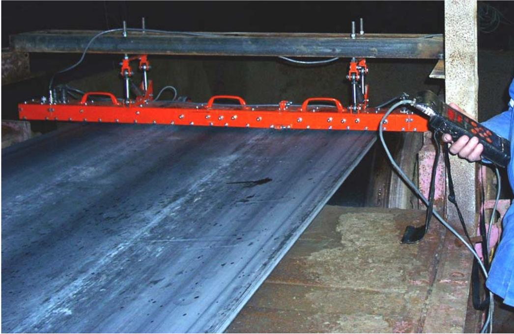
Fig. 1: INTROCON flaw detector on a conveyor.
