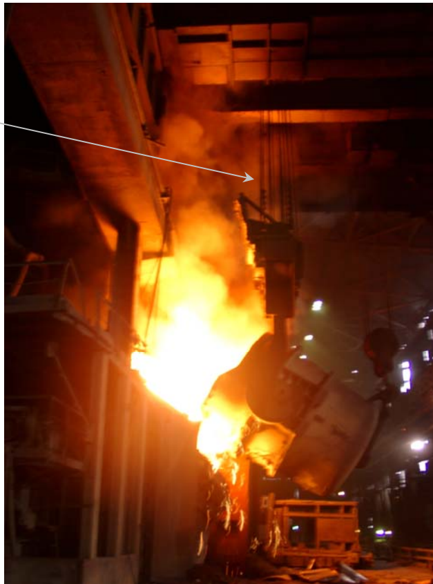
Fig. 1. Pouring of metal into a converter at the SEVERSTAL plant
