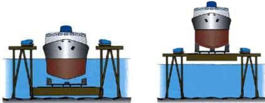
**Figure 6. Scheme of the ship synchrolift**
