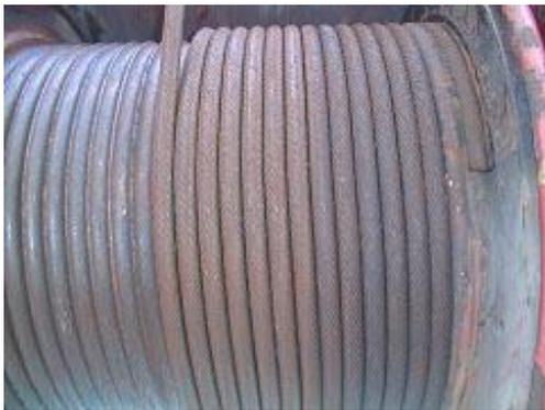
**Figure 2. Lubricated main hoist rope with flight rust on surface**
