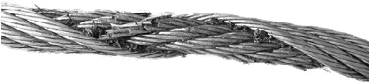
**Figure 3:** Section 1 of the rope A with outer layer strands partly removed.
