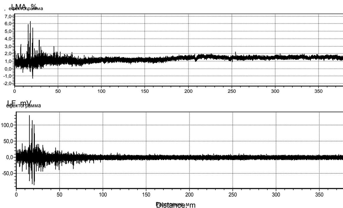
**Figure 1:** Data charts of the crane POTAIN MD-185A loading rope (rope A).
