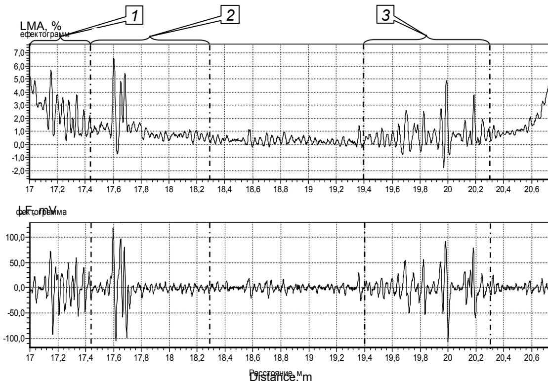
**Figure 2:** LF and LMA traces of the rope A, section 17-21 m.
