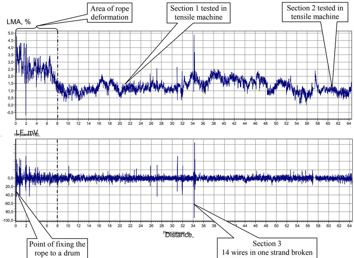
**Figure 4:** Data charts of the crawler crane DEK-251 boom rope (rope B).
