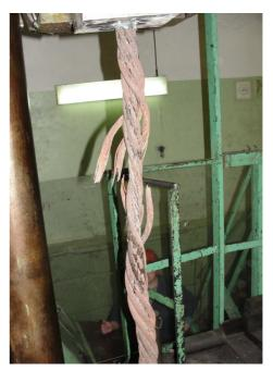
Figure 3: Tensile testing of discarded ladle crane rope.
