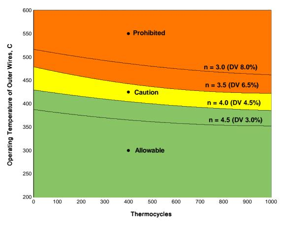
Figure 6: Specific working conditions of wire ropes for ladle cranes at a steel mill.
