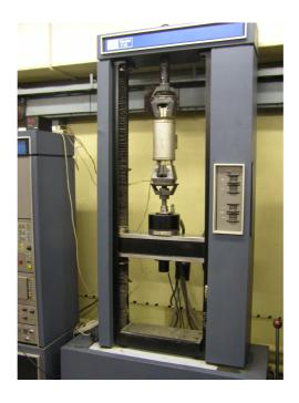
Figure 5: Tensile testing of hot wires.
