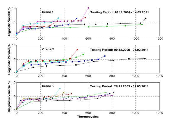
**Figure 2:** Changing of diagnostic variable of hot crane ropes with thermocycles.
