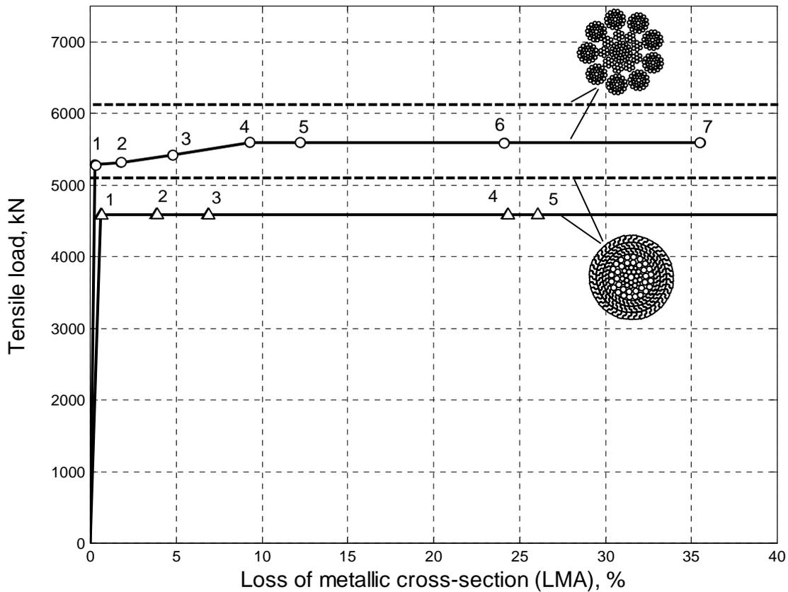
Figure 6: Failure courses of locked coil rope D 72 mm and stranded rope D 84 mm
