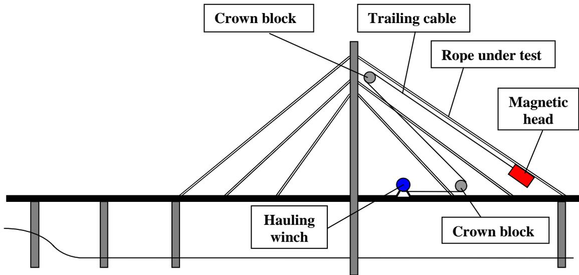
Figure 3: Layout of stay rope diagnostic equipment
