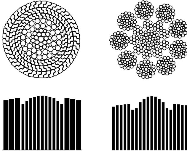
Figure 5: Equivalent stresses over cross-sections for tensed locked coil rope (left) and stranded rope (right)
