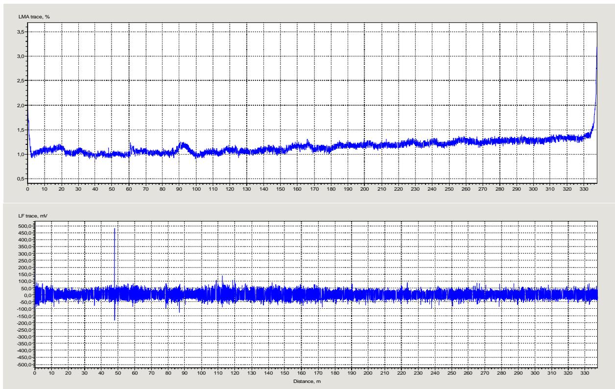
Figure 4: LMA- and LF-traces of stay rope inspection
