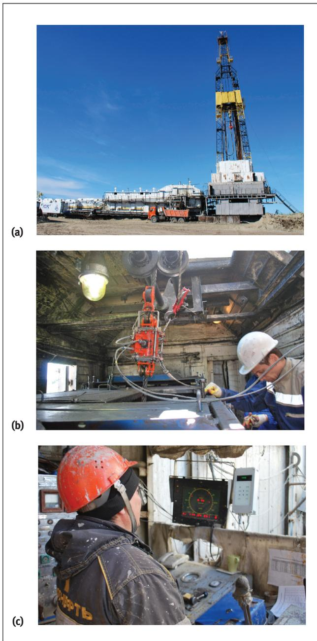
**Figure 3. Rope condition monitoring: (a) drilling rig with calf line under test; (b) the magnetic head on the rope; and (c) the electronic unit in the drilling operator compartment.**
