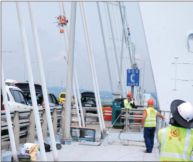
Figure 6. Stay rope testing at the Yeongjong Bridge, South Korea.
