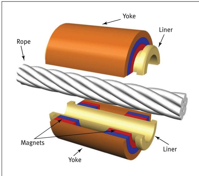
Figure 1. Diagram of a magnetic head for rope testing.
