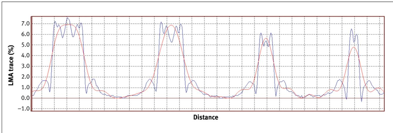
Figure 7. Loss of metallic area (LMA) trace before and after filtering.
