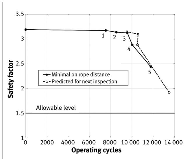
Figure 9. Safety factors and prospective estimates for crane rope.
