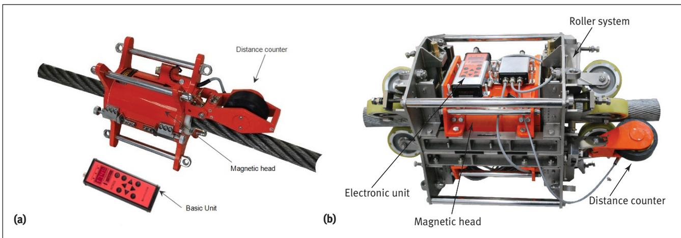
Figure 2. Magnetic flux leakage testing flaw detector design for rope diameter: (a) 20 to 40 mm; and (b) 80 to 120 mm.
