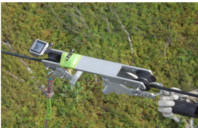
Fig. 2. Video recording device FPV moving system
