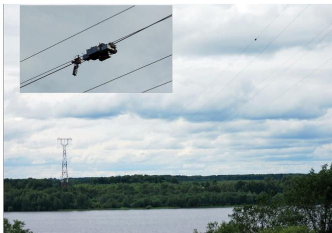
Fig.9. Inspection of the OHL 110 kV «Vichuga - Zavolzhsck» conductors
