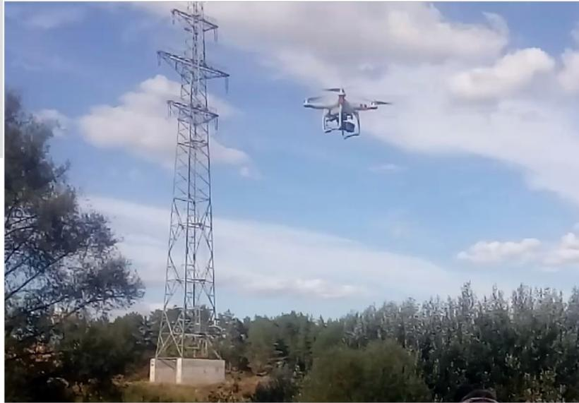
Fig. 1. Monitoring of an OHL 35 kV conductor using an air drone equipped by video recording device
