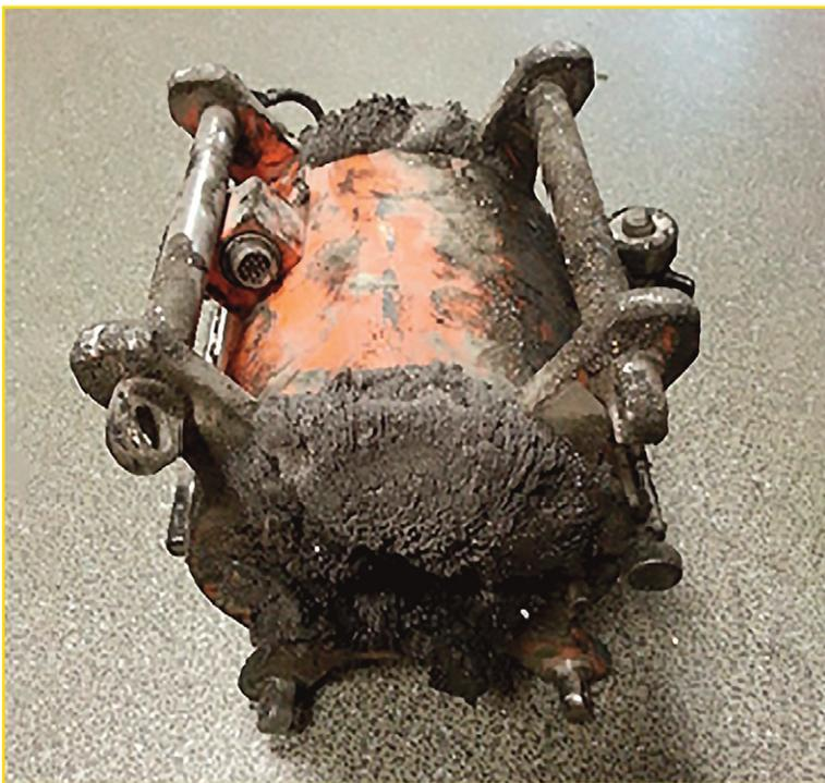
Figure 1. A flaw detector's magnetic head after a single inspection of a crane rope in a metallurgical plant.
