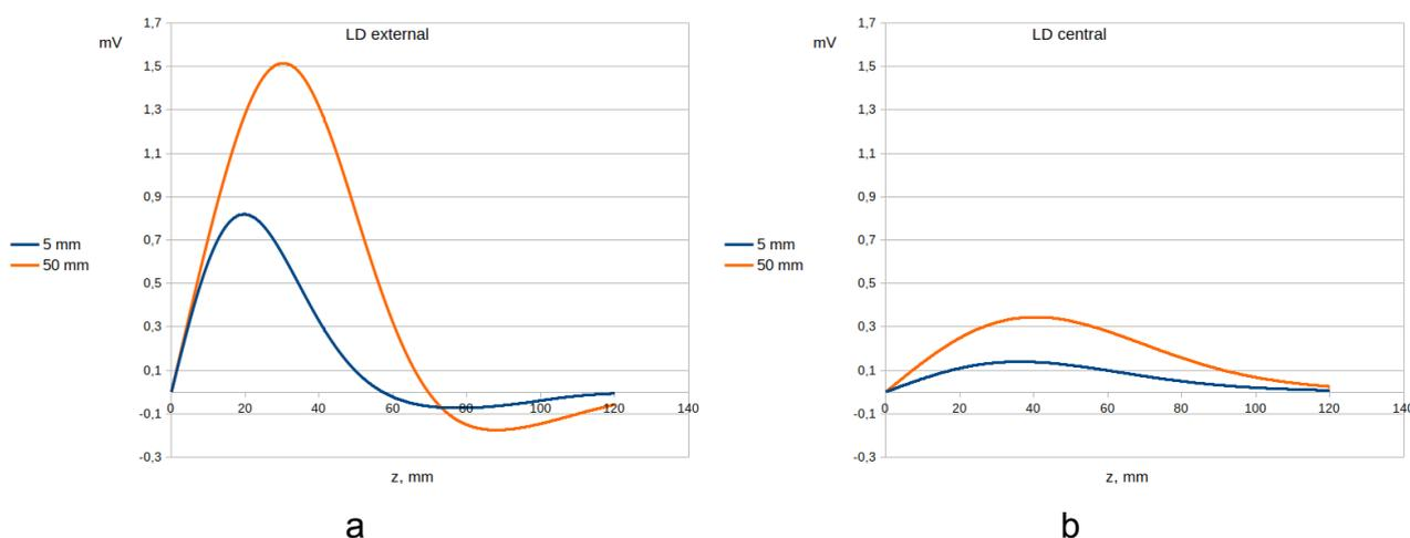
**Figure 3.** Simulated signals from external and internal wire breaks for normal magnetization
