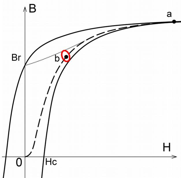
Figure 2. Rope magnetization curve
