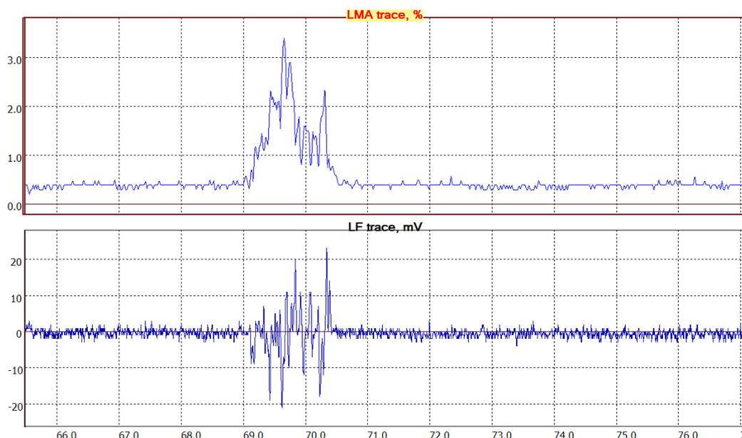
**Figure 5.** LMA and LF traces of a cluster with 13 wire breaks
