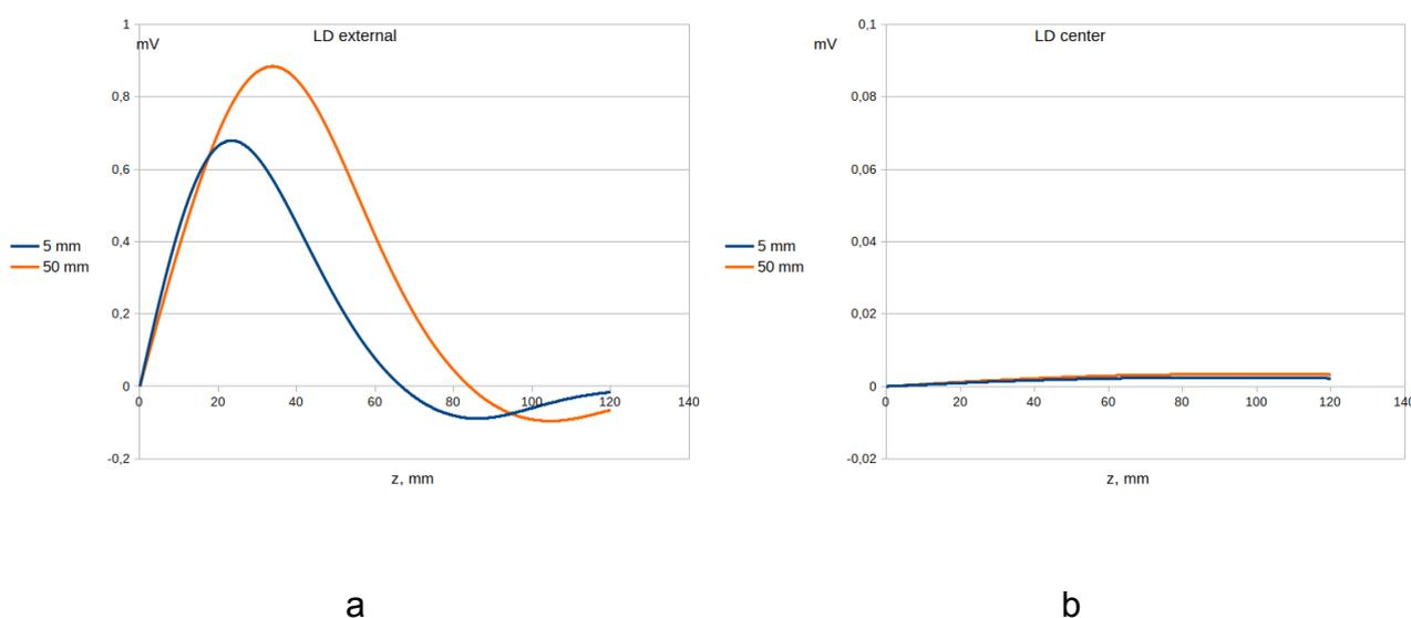
**Figure 4.** Simulated signals from external and internal wire breaks for low magnetization
