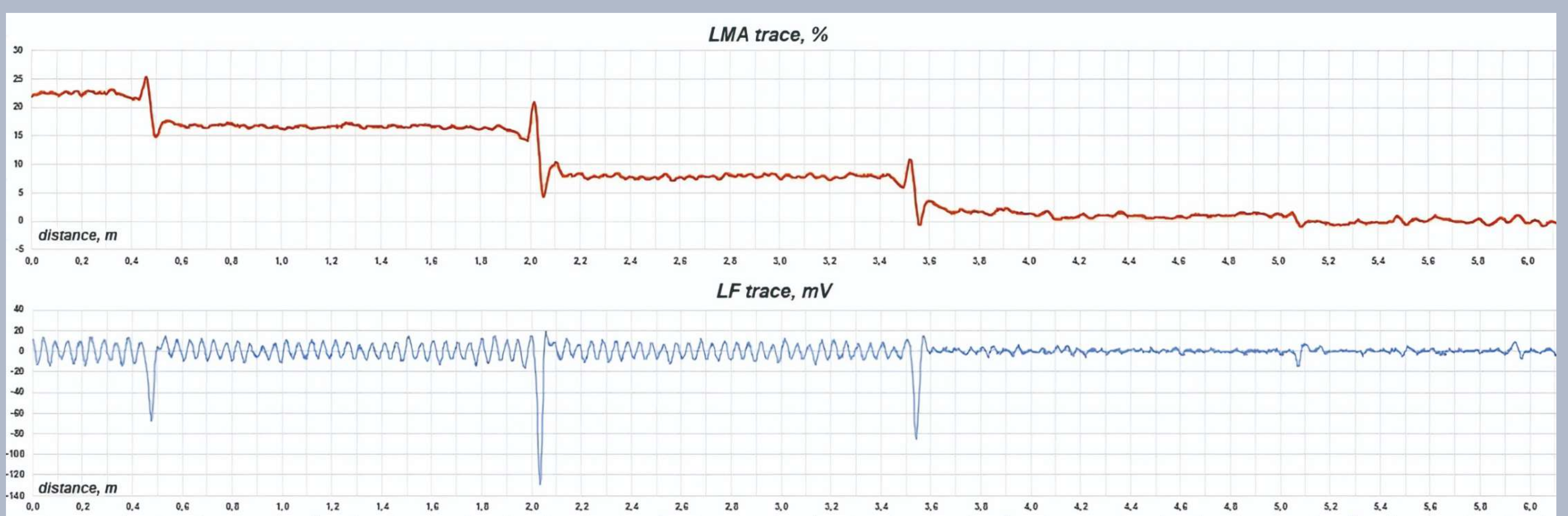
Example of data obtained during inspection of 24 mm diameter wire rope with the local faults
