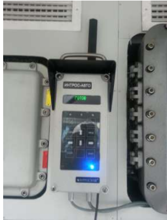
Figure 2. Control and display unit of Intros-Auto at operator console
