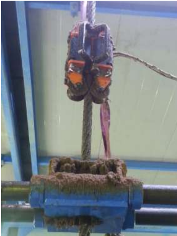
Figure 1. Magnetic head of Intros-Auto at the rope
