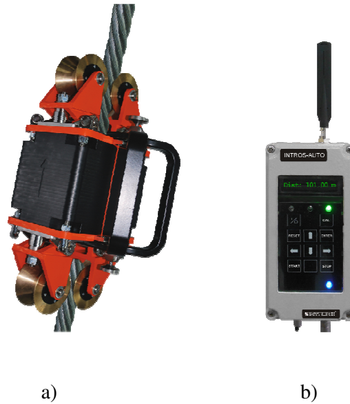
Fig.4. INTROS-AUTO consists of magnetic head (a) and CDU (b)
