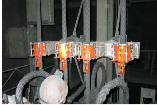
Fig.6. System INTROS to simultaneously inspect 4 mining ropes.
