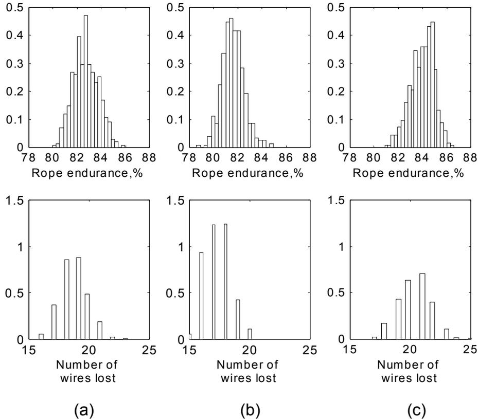
**Figure 1:** Histograms of damaged rope parameters for different initial failure probabilities of the wires:  $P_i = \text{const}$ (a),  $P_i \sim A_i$ (b),  $P_i \sim 1/A_i$ (c).
