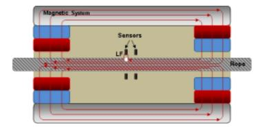
Fig. 1, MFL principle of operation.
