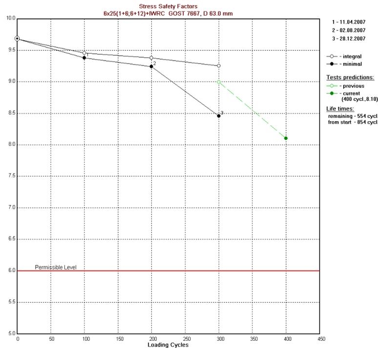
Figure 4. Degradation of safety factor of the shaft rope with operating time
