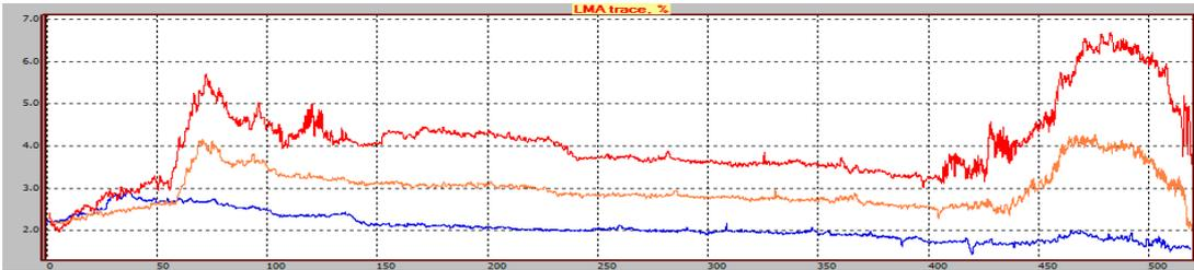
Figure 1 LMA-distributions of the shaft rope during three consecutive inspections
