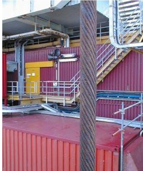
**Figure 3. Rope segment above the crane hook with corroded outer strands**
