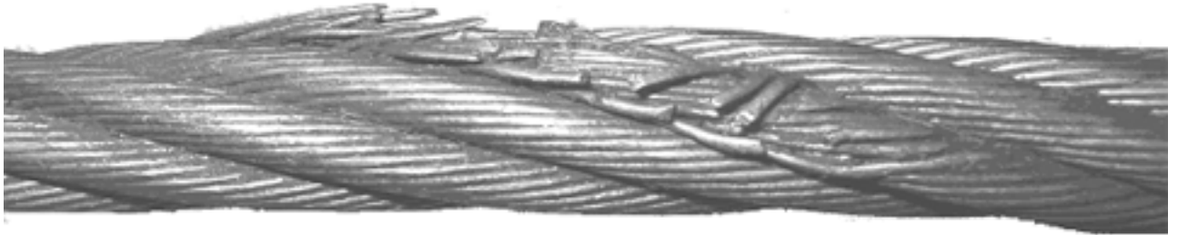
Figure 5: Wire breaks of the rope B one strand (section 3 in Figure 4).
