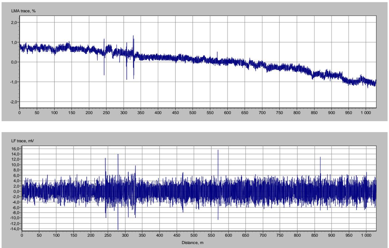
Fig. 6. LMA and LF charts of rope 38,5 mm. Charts obtained by INTROS rope tester.
