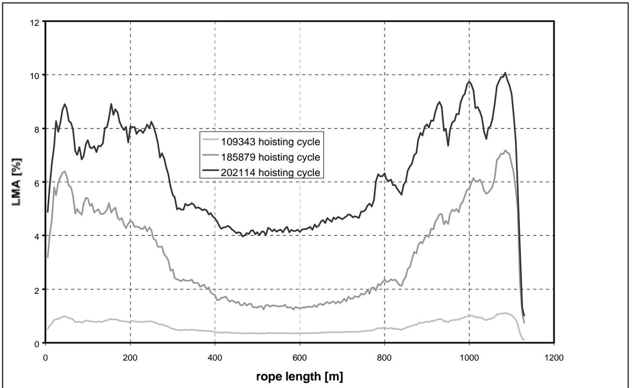
Fig. 4. LMA traces obtained from the rope after different hoisting cycles
