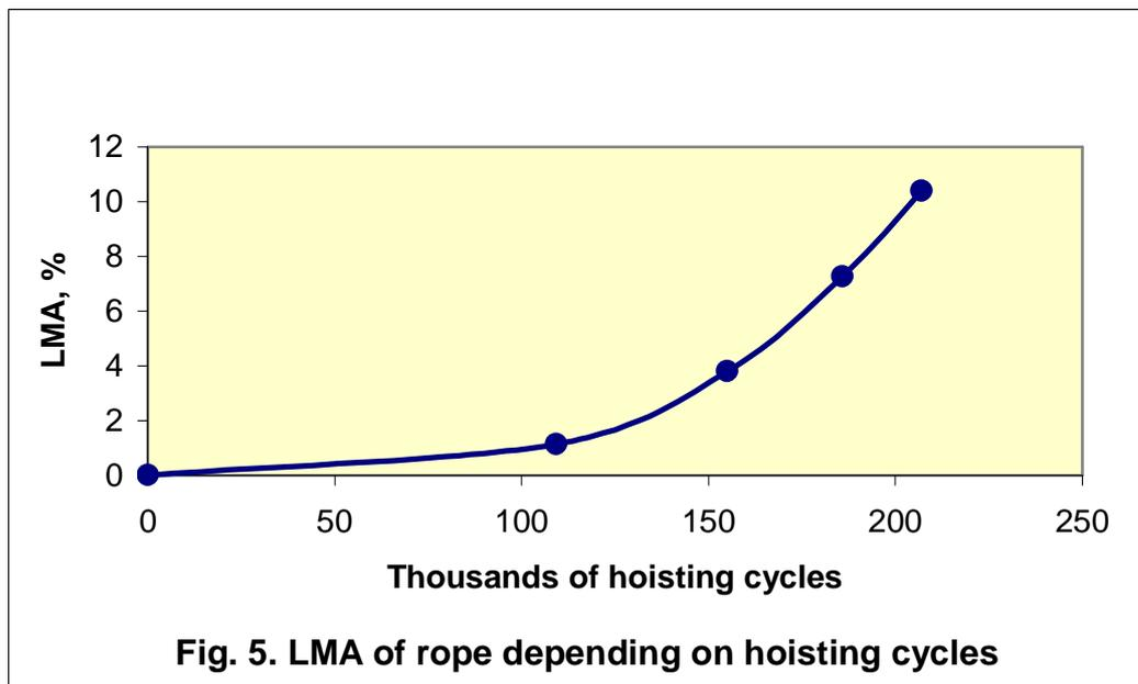
Fig. 5. LMA of rope depending on hoisting cycles
