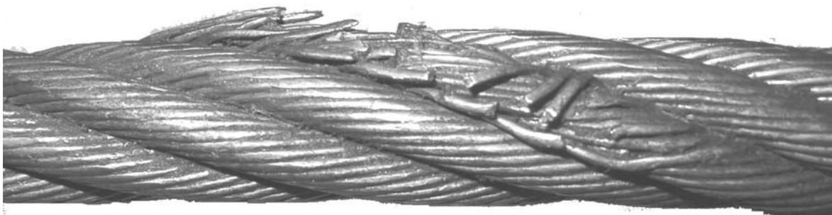
**Figure 5:** Wire breaks of the rope B one strand (section 3 in Figure 4).
