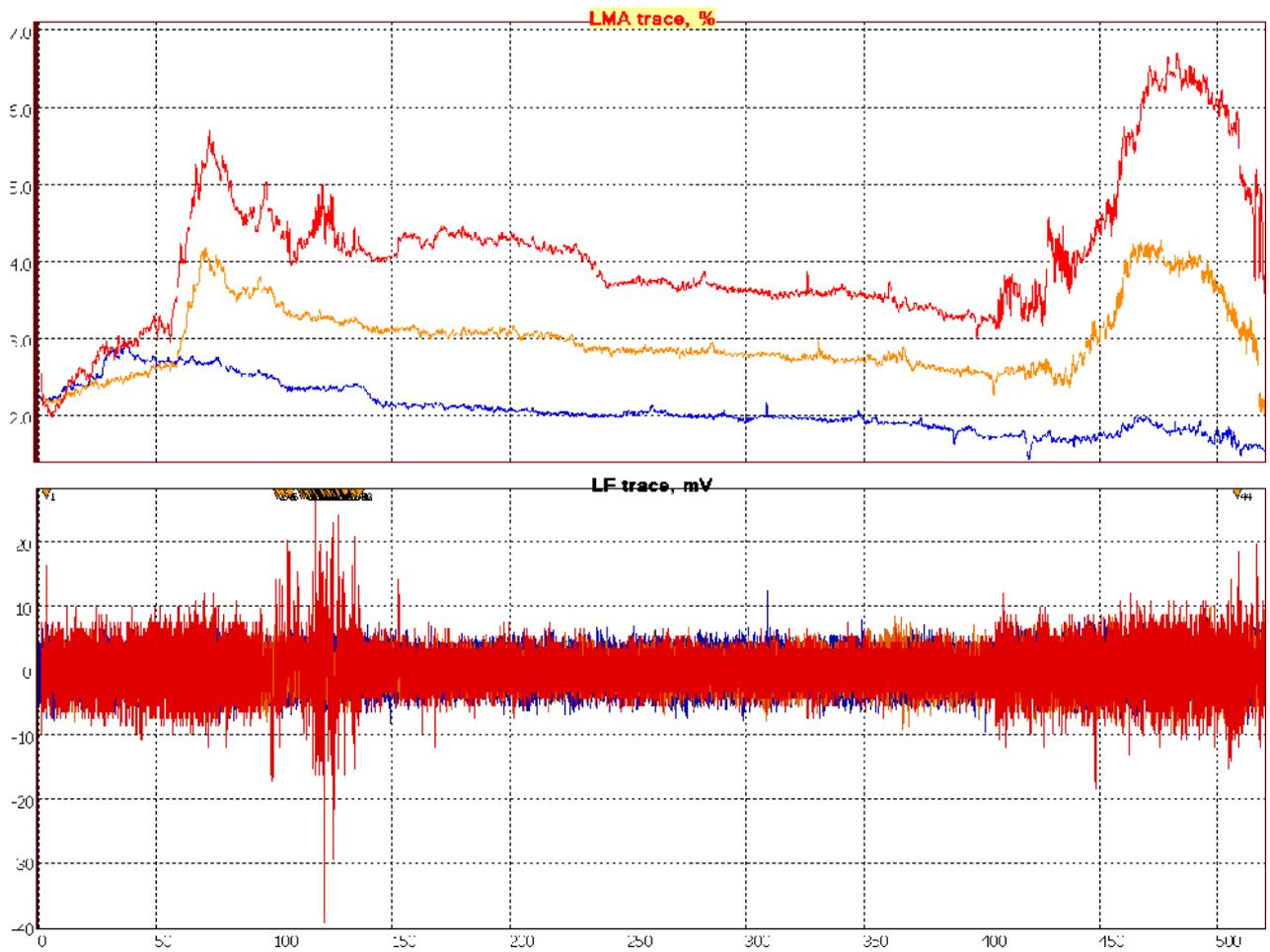
Figure 1. Distribution of LMA and LF of the shaft rope during 3 consecutive inspections.
