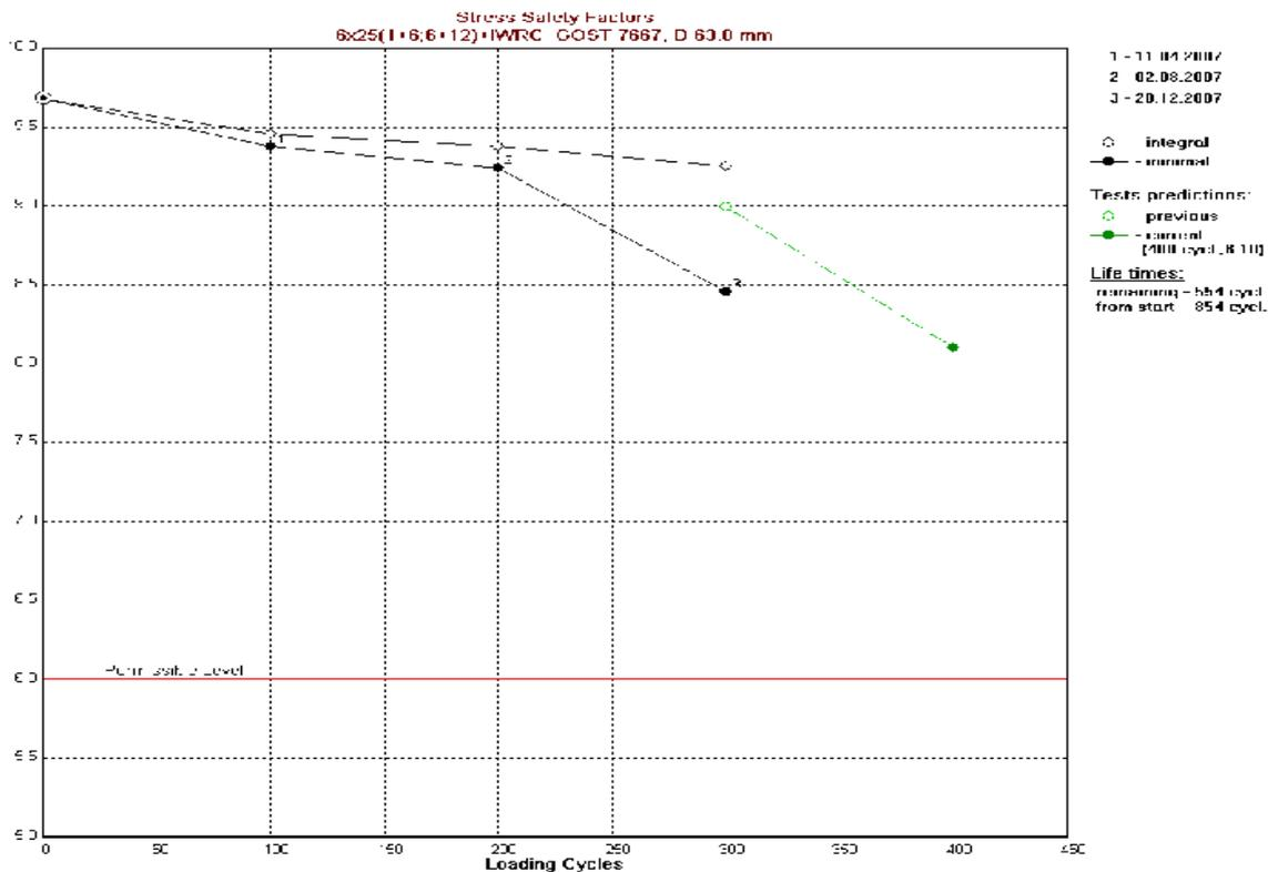
Figure 4. Degradation of Safety Factor of the shaft rope with a time.
