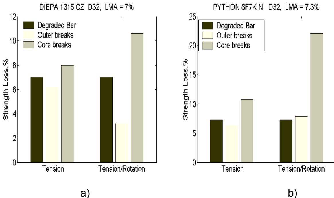
Figure 3 Strength loss depending on failure location and operating condition
