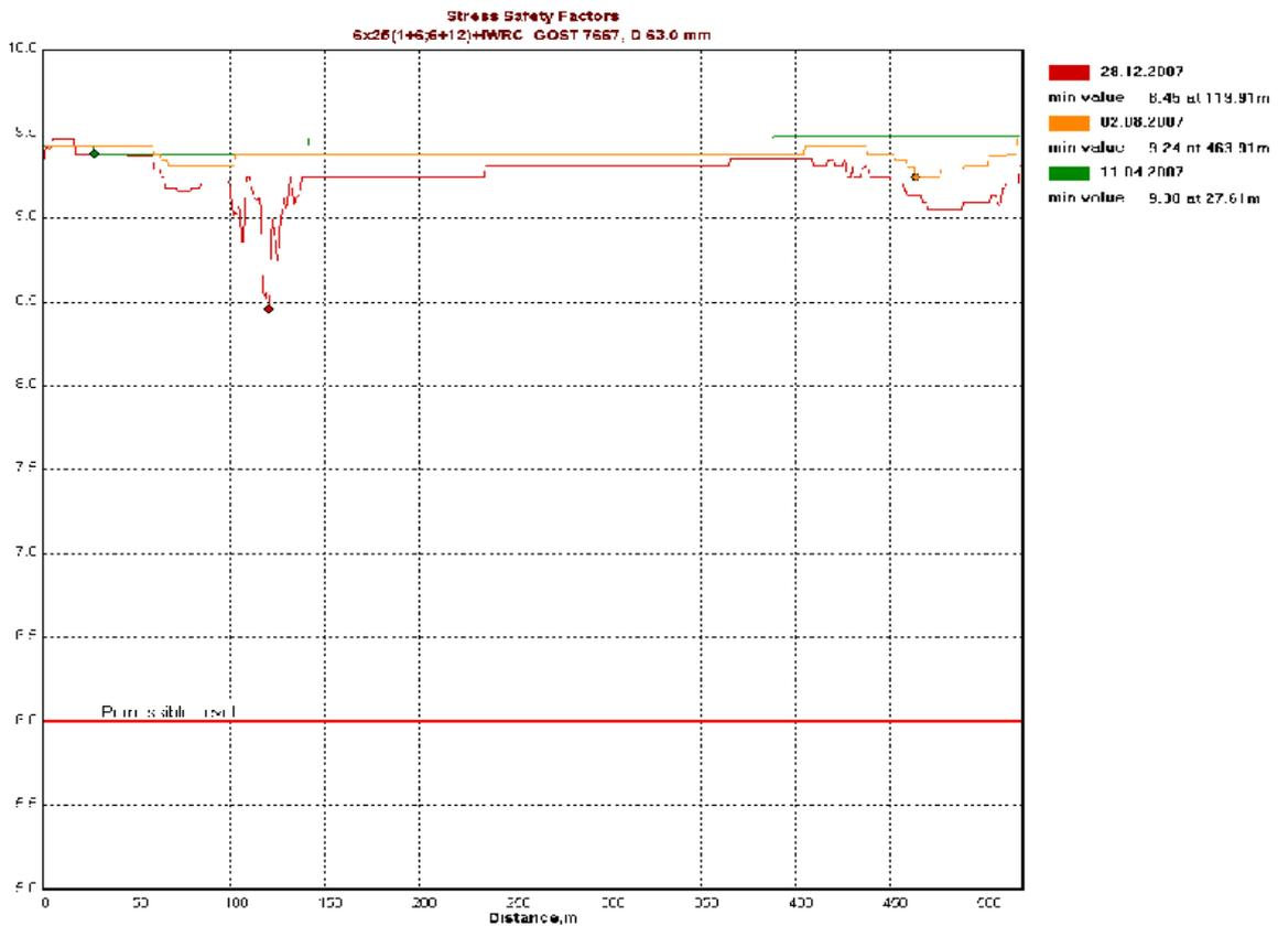
Figure 2. Distribution of Safety Factor of the shaft rope during 3 consecutive inspections.
