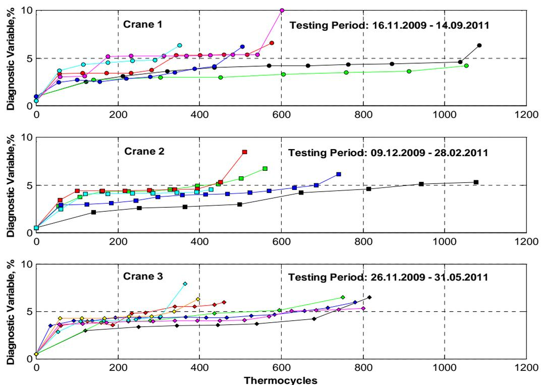
Figure 2: Changing of diagnostic variable of hot crane ropes with thermocycles.
