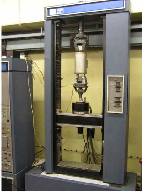
**Figure 5:** Tensile testing of hot wires.
