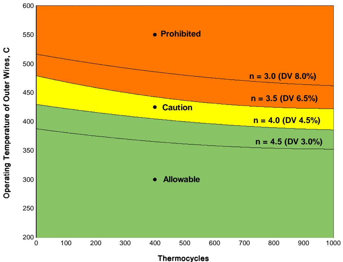
Figure 6: Specific working conditions of wire ropes for ladle cranes at a steel mill.
