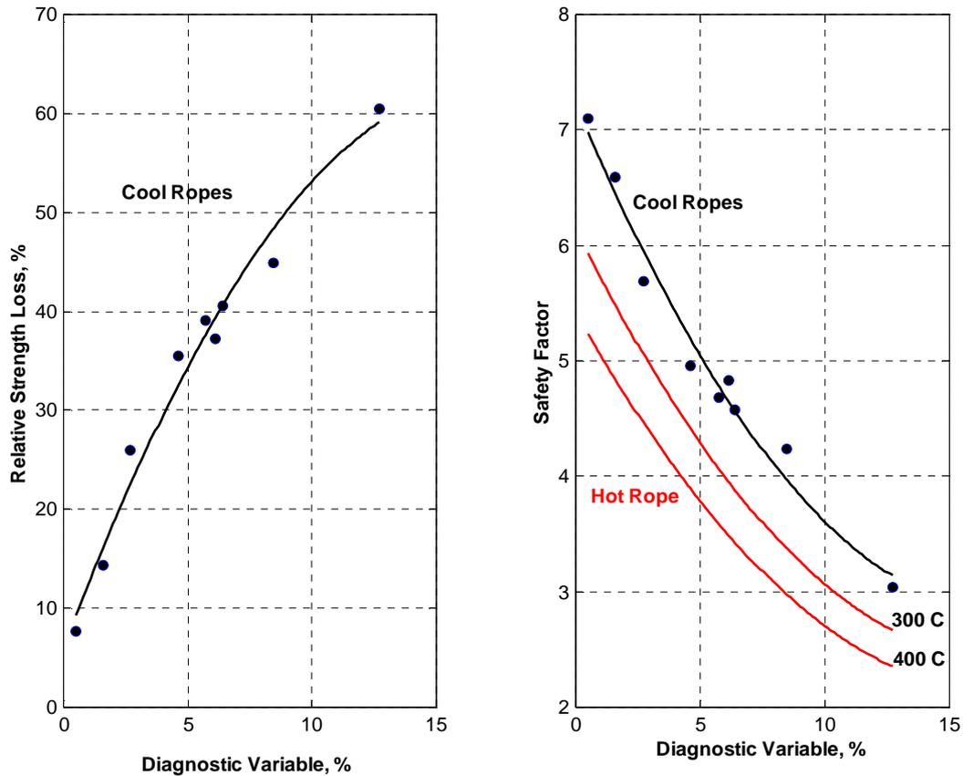
**Figure 4:** Strength parameters of hot metal crane ropes as functions of diagnostic variable.
