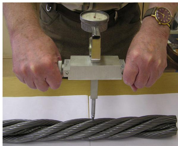
**Figure 7:** Hardness testing of worked-out ladle crane rope.
