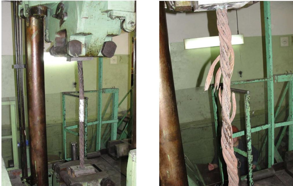
**Figure 3:** Tensile testing of discarded ladle crane rope.
