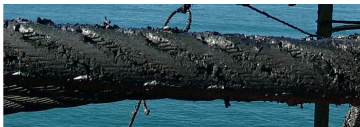
Figure 1. Cross section of multilayer rope (left) and heavy greased crane rope (right).
