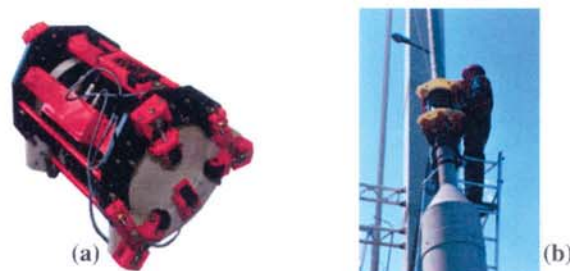
Figure 3: Electromagnetic head EH-300 (a) and testing of EH-300 at the bridge cable (b).
