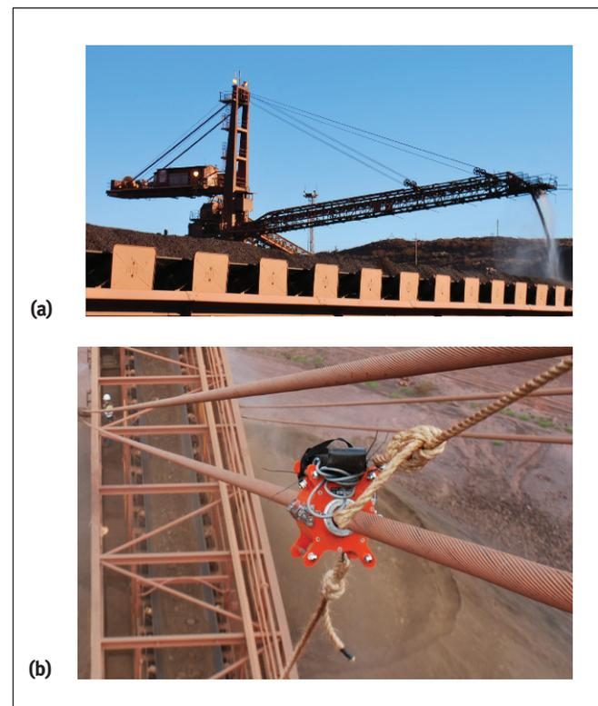
Figure 5. Rope testing in Paraburdoo, Australia: (a) the commercial stacker being tested; and (b) magnetic head on the rope.
