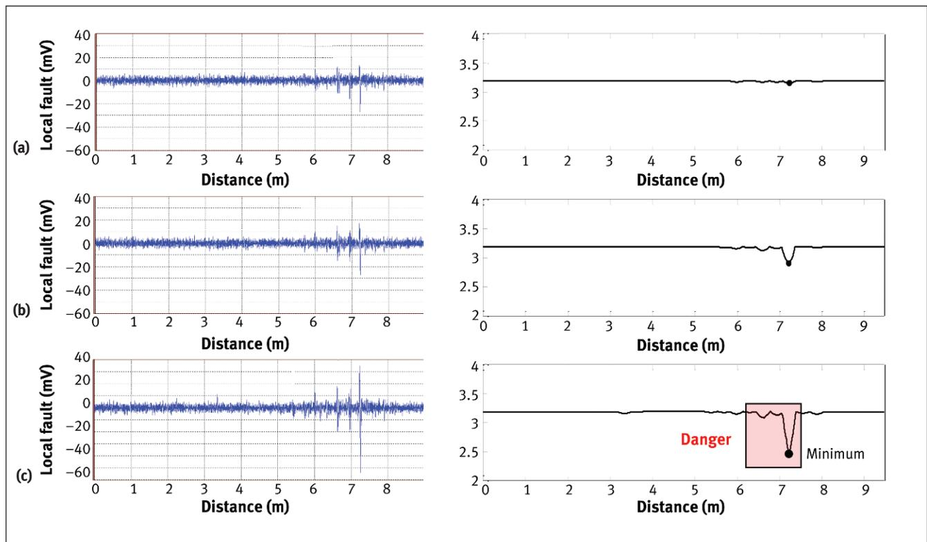
Figure 8. Local fault charts and distributions of crane rope strength parameter: (a) in June 2007; (b) in October 2007; and (c) in November 2007.
