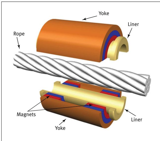
Figure 1. Diagram of a magnetic head for rope testing.
