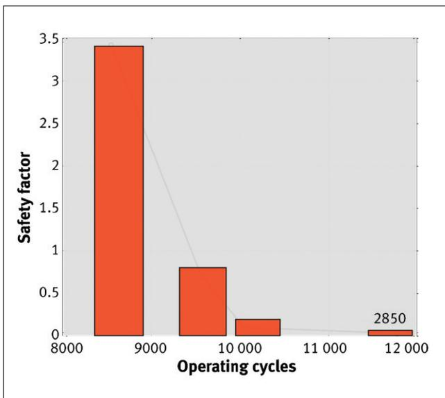
Figure 10. Remaining lifetime estimates for crane rope.
