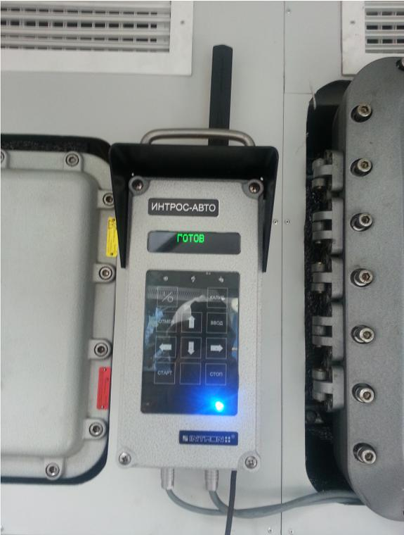
Figure 2b. Control and display unit of Intros-Auto at operator console
