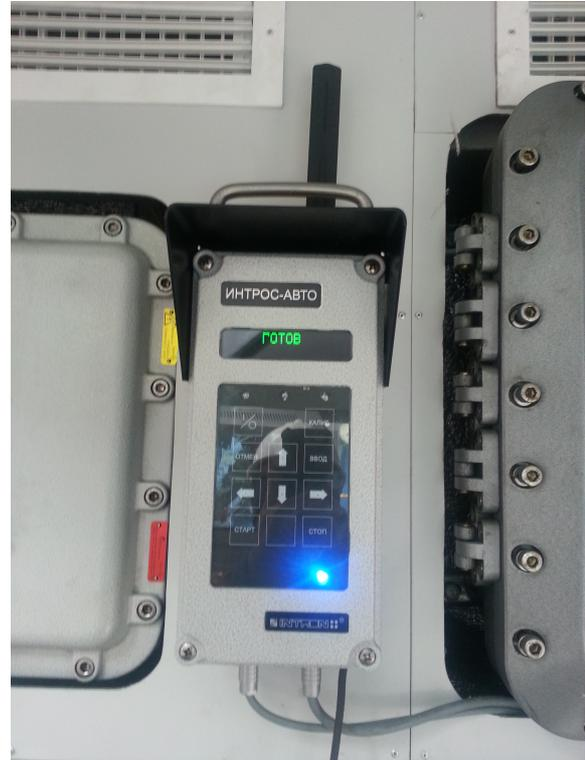
Figure 2b. Control and display unit of Intros-Auto at operator console
