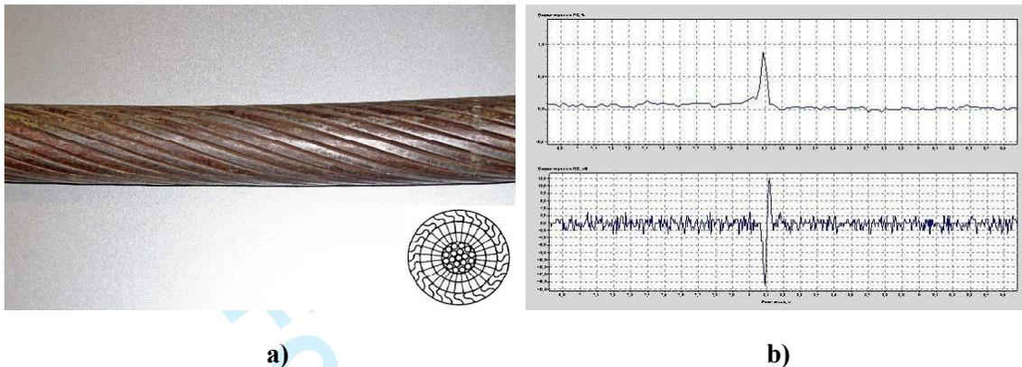
**Figure 2. (a) Locked rope and LMA and (b) LF traces for its part containing a broken wire**
