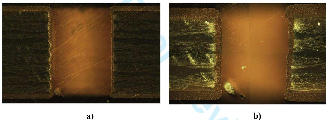
**Figure 1. Microsection of the PCB's 1.1 mm diameter through hole with copper coating inside: a) overview; b) four zones of the section adjacent to PCB's surfaces composed in one picture and enlarged 2.5 times to picture (a). Maximal and minimal values of coating differ each other more than five times, standard deviation is 14%**
