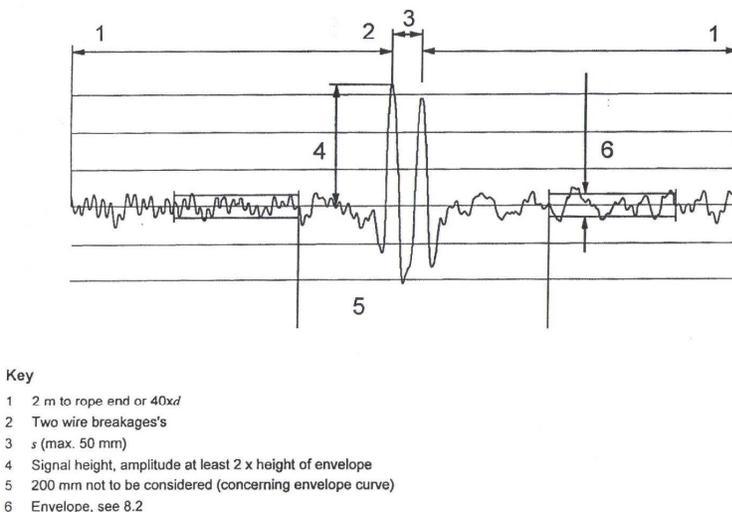
**Figure 5. Trace of the LF performance test according to EN 12927 - 8**
