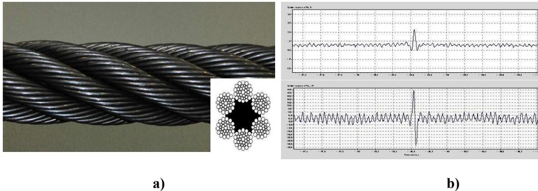
**Figure 4. (a) Strand rope and (b) the traces for its part with a broken wire**
