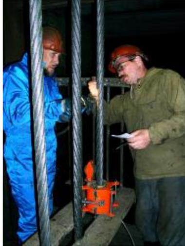
Fig.2. Visual examination of suspected part of rope right after instrumental inspection by rope tester INTROS
