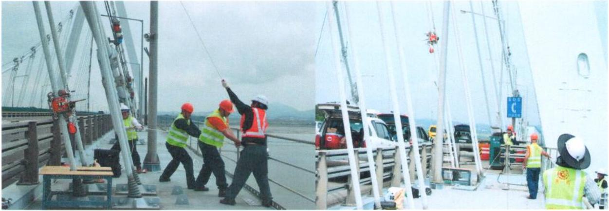
Fig. 17: Stay ropes testing at bridge: (a) by hand pulling; (b) by winch pulling.
