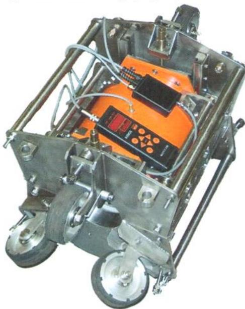
Fig. 6: Magnetic head with a roller system and a basic unit.
