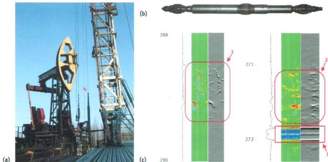
Fig. 10: NDT of an oil well pipe casing by the INTROSCOPE tool (a) the tool (denoted by an arrow); (b) the tool view; (c) data records showing: 1-corrosion damage of casing external surface; 2- corrosion damage of casing internal surface and 3- perforation.
