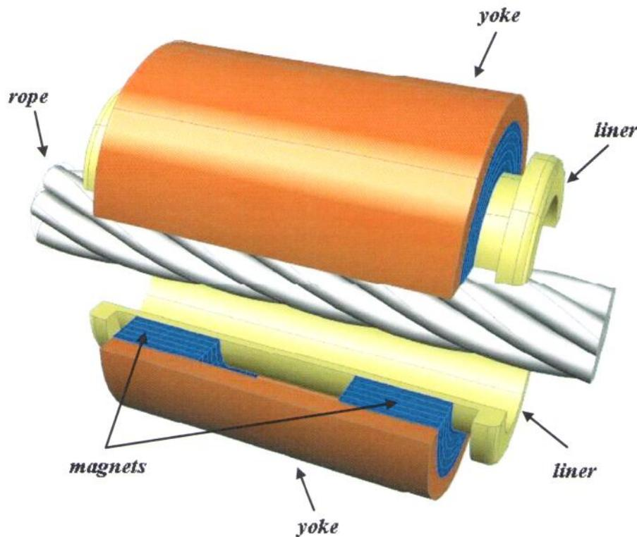
Fig. 5: Diagram of magnetic head for rope testing.
