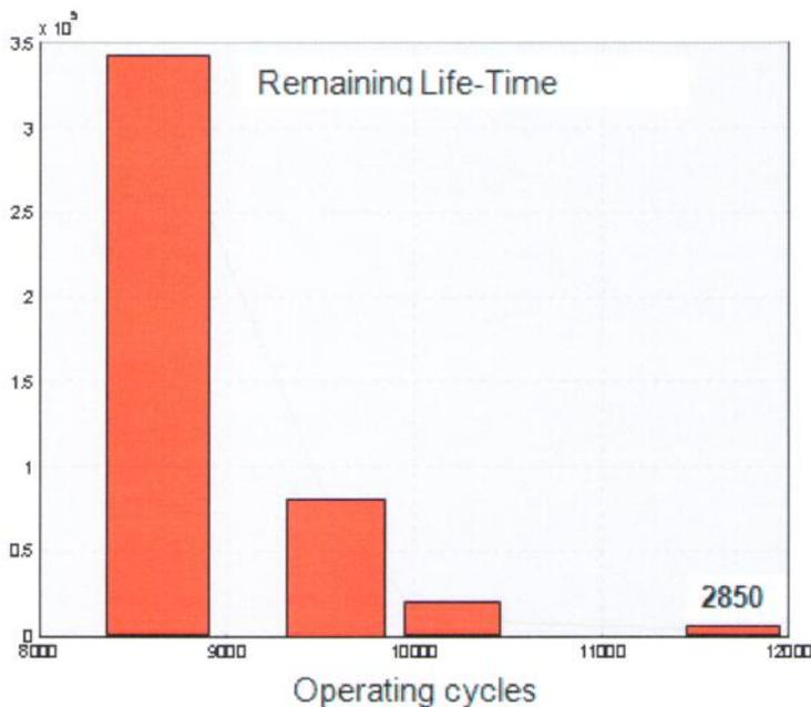
Fig. 13. Remaining life-time estimates for crane rope PYTHON D8
