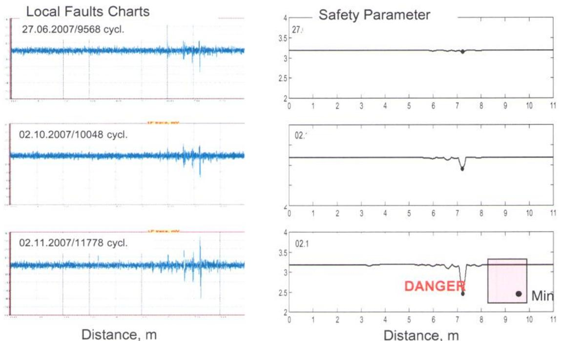
Fig. 11. LF-charts and distributions of crane rope PYTHON D8 strength parameter
