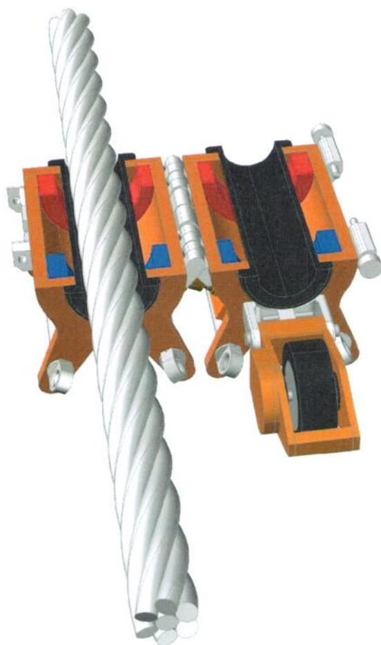
Fig. 1: Magnetic head opened with a rope.
