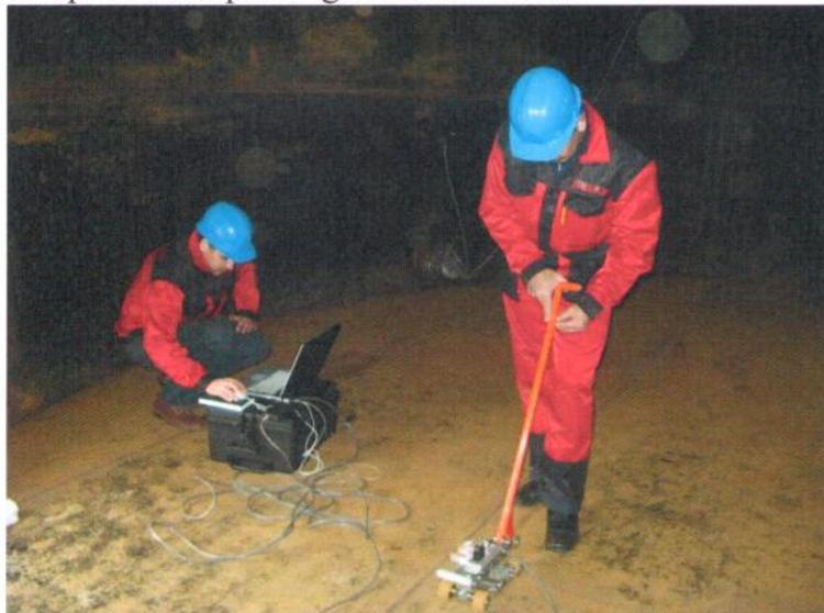
Fig. 8: The INTROCOR scanner with scan width 150 mm
