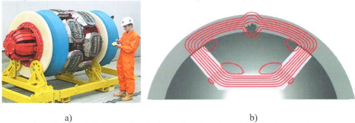
Fig. 9: The ROSEN RoCorr.CMFL taken for pipe axial flow detection: the tool view (a) and the diagram of magnetic flux (b).
