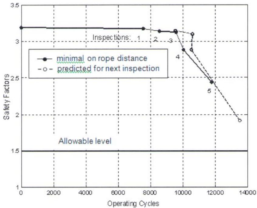
Fig. 12. Safety factors and prospective estimates for crane rope PYTHON D8
