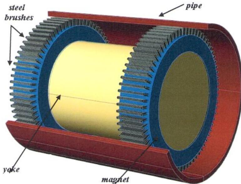
Fig. 2. Diagram of a PIG magnetic system.
