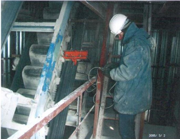
Fig. 14: Inspection of a flat steel-rubber rope by the INTROS instrument.
