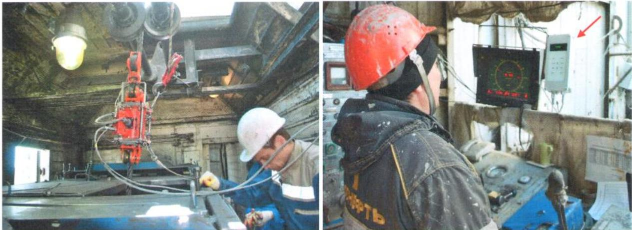
Fig. 7: The INTROS-AUTO instrument for rope condition monitoring:
