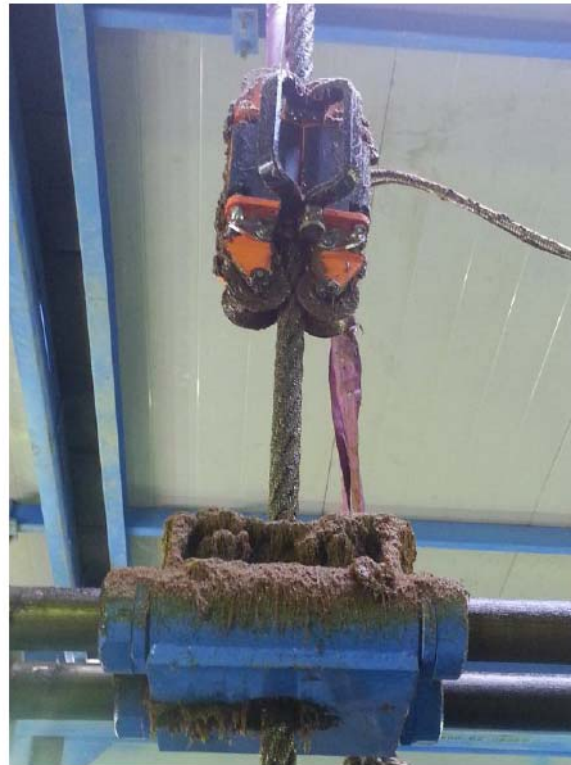
Figure 3: MH of Intros-Auto at the 28-mm rope of the drilling rig
