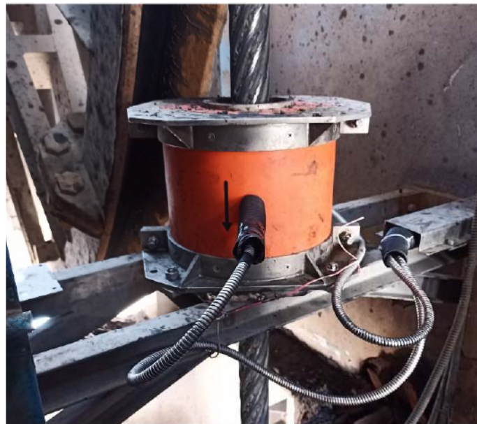
Figure 1: Magnetic head of Intros-Auto at the 56-mm rope of the mine hoist.
