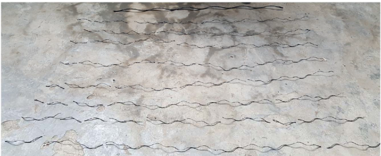
Figure 4: Disassembled section of the automatically discarded rope
