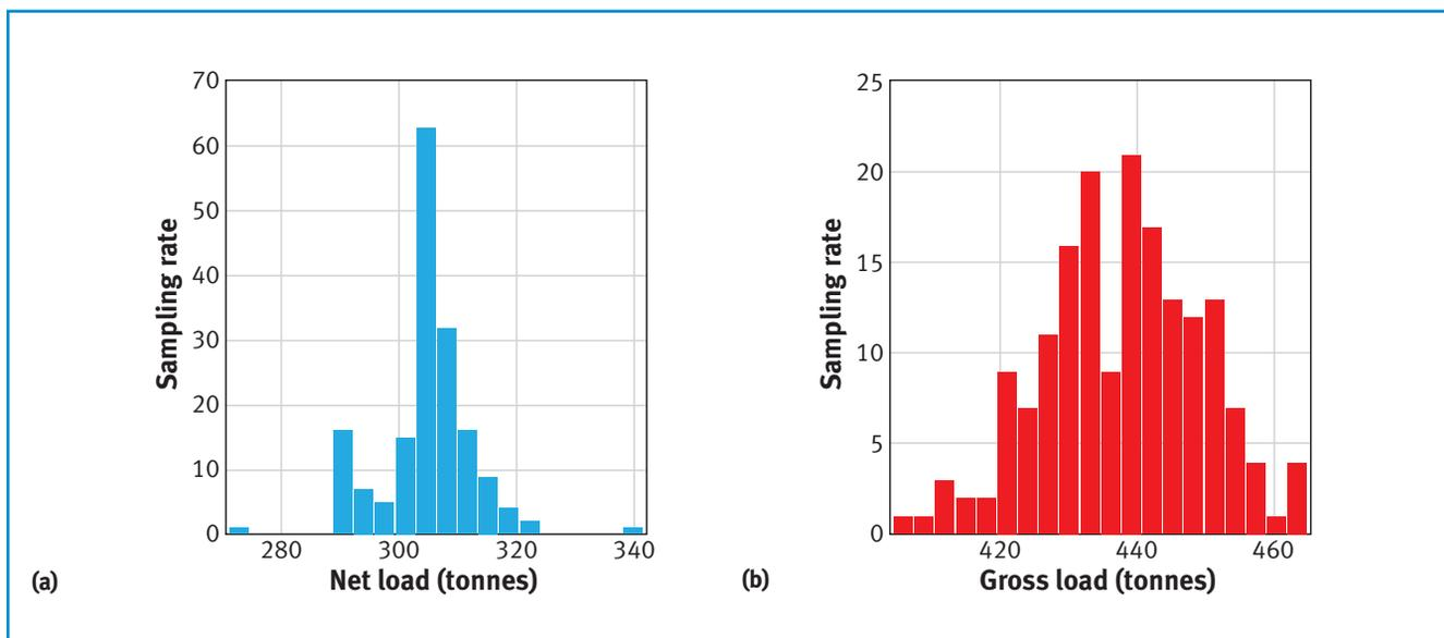
Figure 2. Histograms displaying the loads on ladle ropes: (a) net load; (b) gross load.
