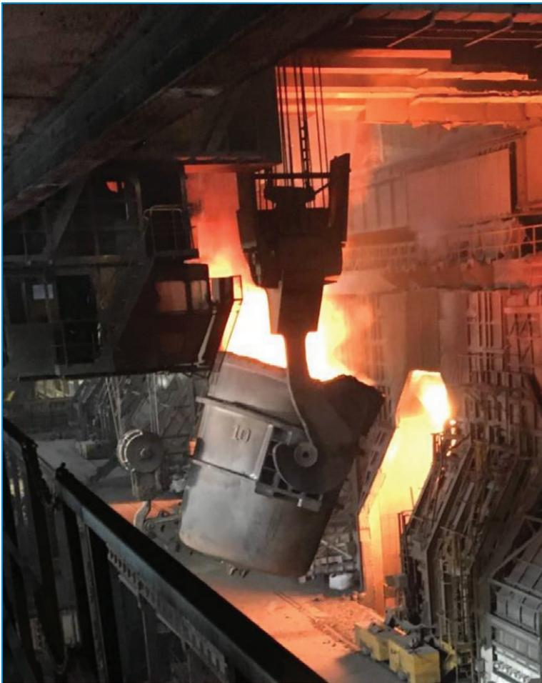
Figure 1. A ladle pouring molten pig iron into a converter.
