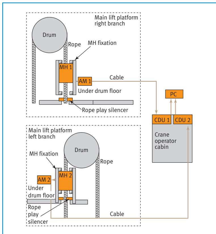
Figure 6. Installation schematic of the automated condition monitoring system for ladle crane ropes (MH = magnetic head; AM = analog module).
