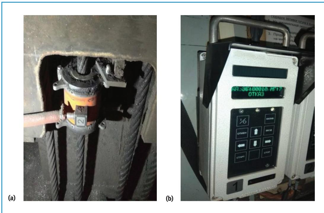
Figure 7. Components of the automated condition monitoring system: (a) magnetic head permanently installed on the rope; (b) control and display unit in the cabin of the crane's operator.
