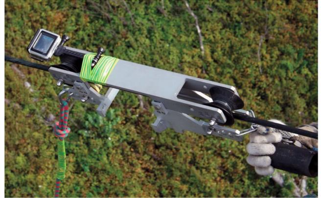
**Fig. 2.** Wheeled system carrying camera along conductors/ground wires.
