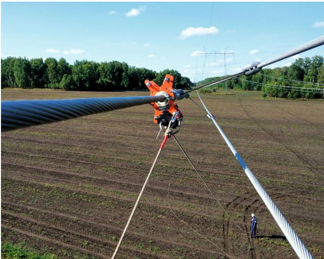
Fig. 4. Pulling of a measuring head with a synthetic rope along a conductor.
