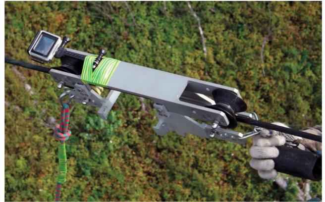
**Fig. 2.** Wheeled system carrying camera along conductors/ground wires.
