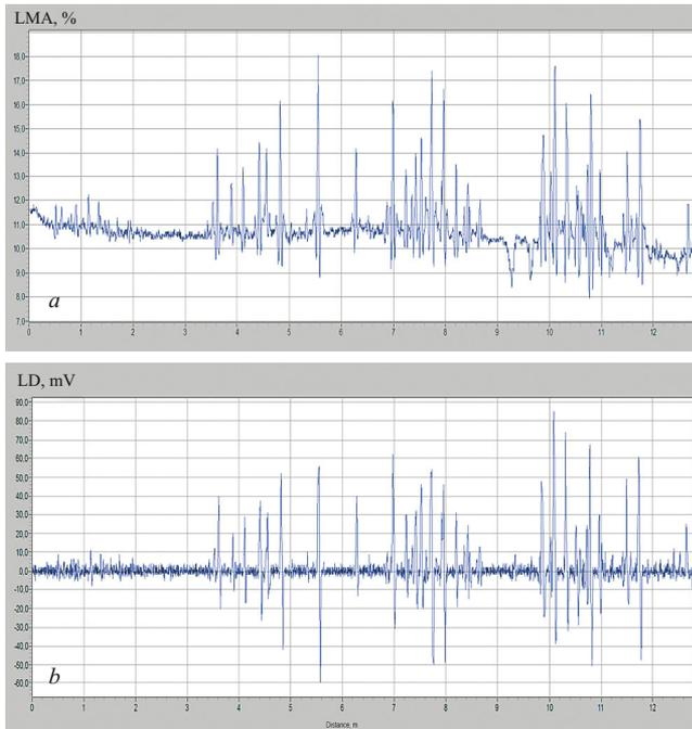
**Fig. 6.** Chart recordings from LMA (*a*) and LD (*b*) channels for the core of BS 185/43 steel-bronze conductor.
