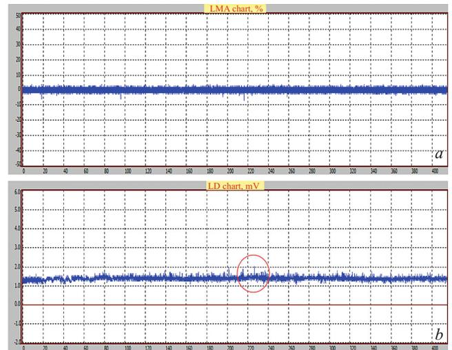
**Fig. 9.** LMA (a) and LD (b) chart recordings for the core of the lower conductor of the Kudelinskaya – Shubinskaya 110 kV OHL crossing (the span between towers 46 and 45) of the Ob' River.
