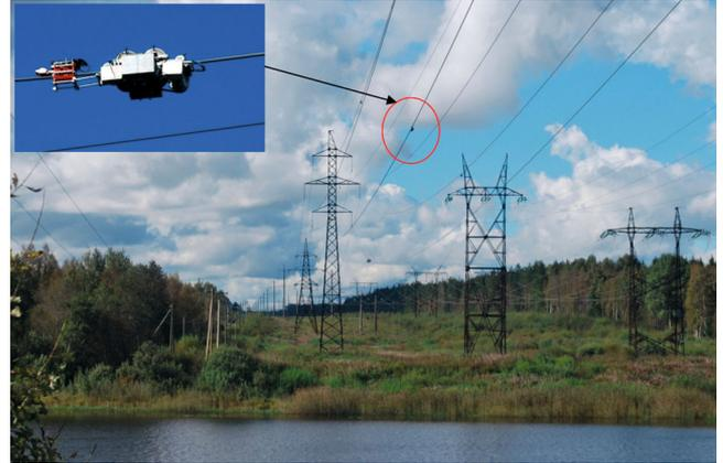
Fig. 5. Self-propelled stand-alone device carrying the measuring head along a conductor.
