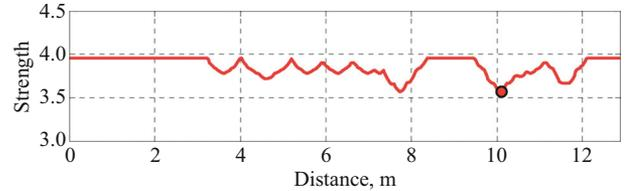
**Fig. 7.** Distribution of strength along BS 185/43 conductor segment.
